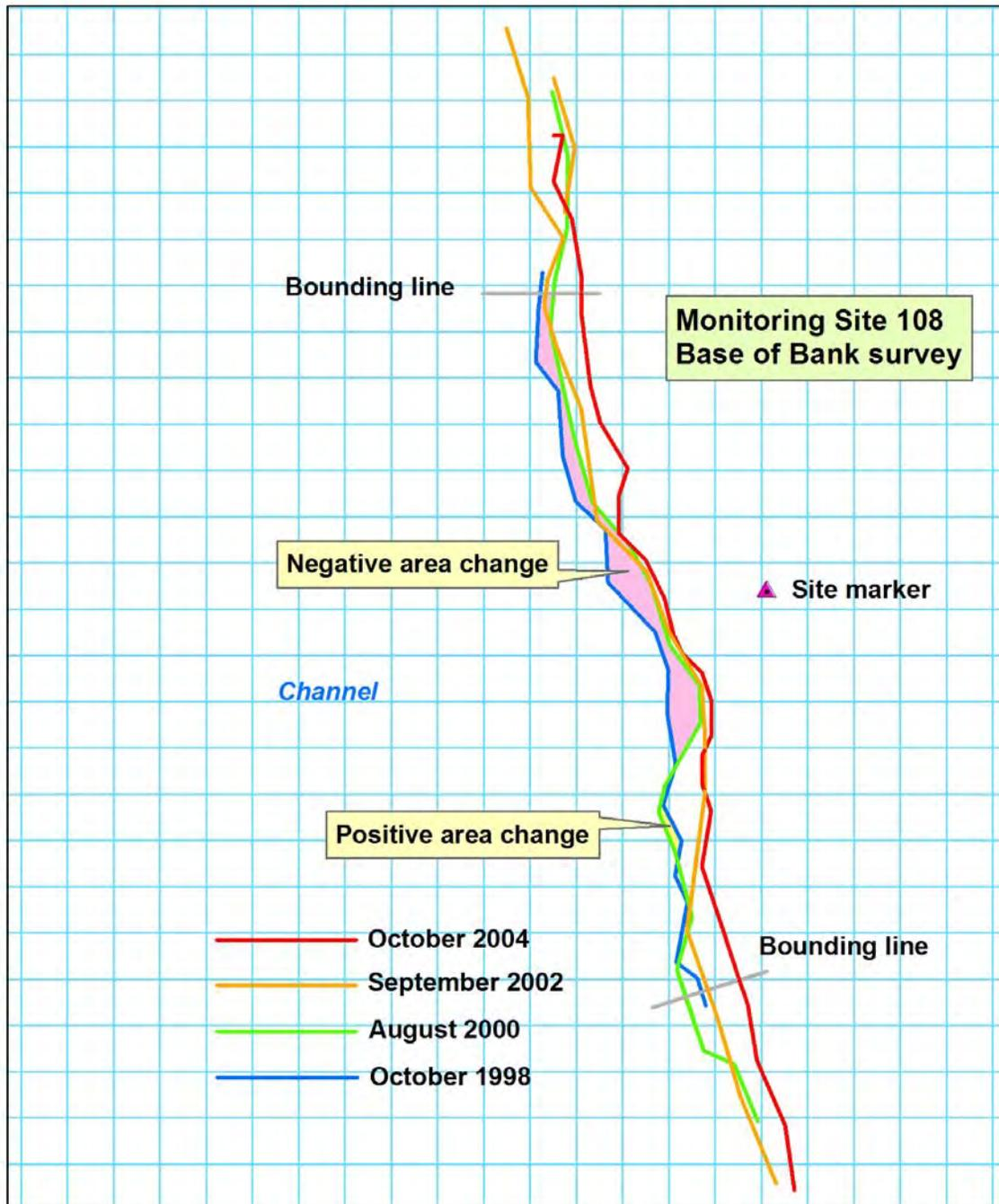
**Figure 4.** Example of change analysis on datasets representing the base of bank for site 108. Lines representing the position of the base of bank during the time of each survey are shown in different colors. A negative change is where the line retreats from the channel, and a positive change is where the line advances toward the channel since the previous survey. The blue grid has 5-foot cells.
