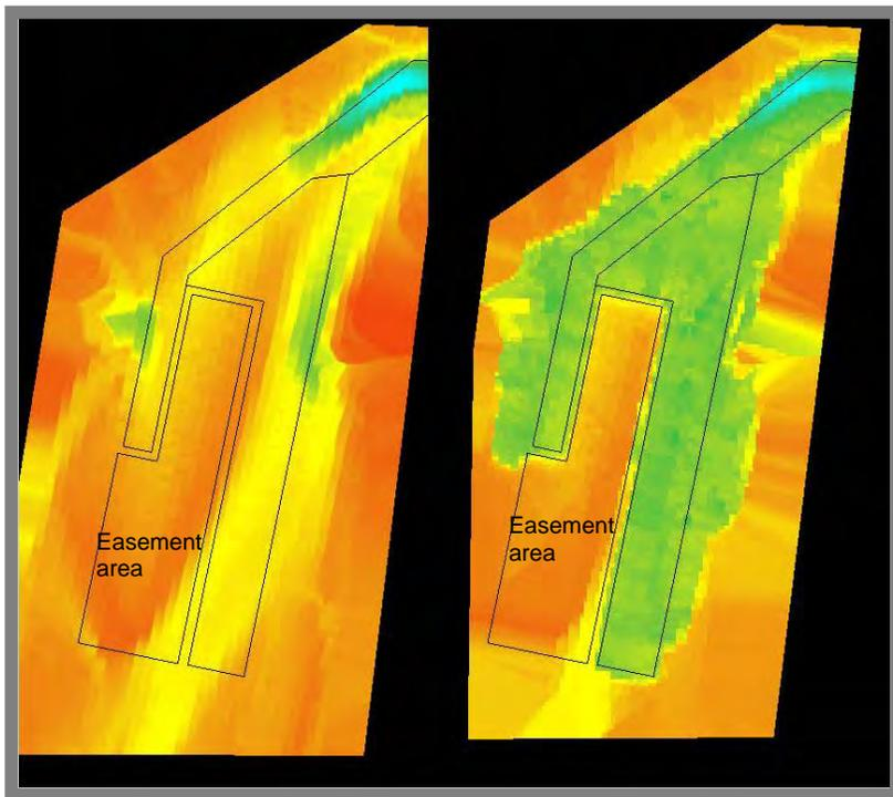
**Figure 2.** Wells Harbor bathymetry before (left) and after (right) dredge. Oranges and yellows are shallow areas, greens and blues are deep areas. The easement area on the flood tidal sandbar is shown, as are the outlines of the federal navigation project.
