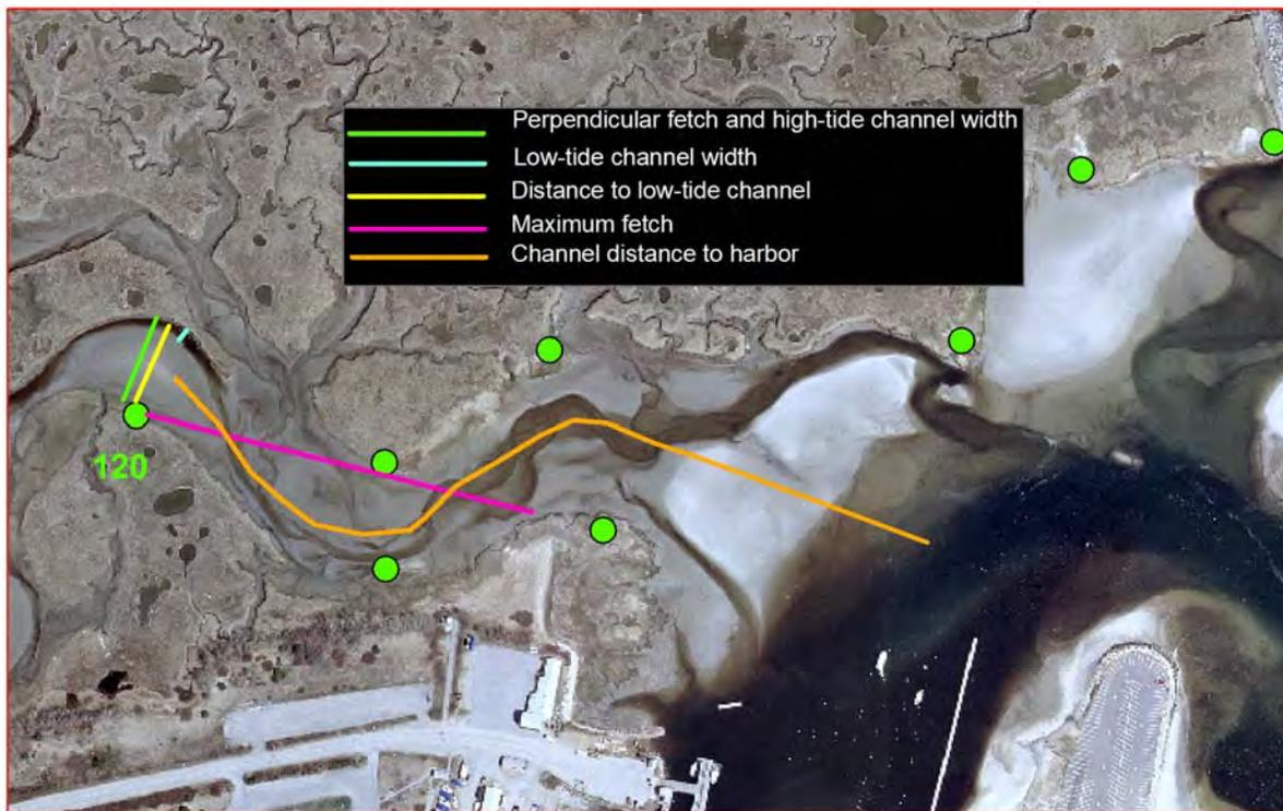
**Figure 5.** Example for Site 120 of measurements made at each site using Spring 2003 one-foot resolution digital imagery and ArcMap software. Distances were measured in meters using the ArcMap measuring tools. Fetch azimuths were determined directly from the image. North is at the top.
